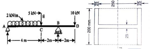
Beam has H cross-section as shown in adjacent figure where dimensions are in mm. Draw the shear stress distribution diagram for a cross-section located at 3.0 m from the left support. Show minimum four stress values between neutral axis and top or bottom surfaces. **06M**
