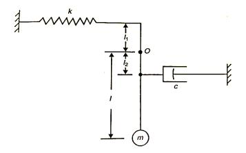
Where m, c and k are the mass, damping coefficient and spring stiffness respectively.
