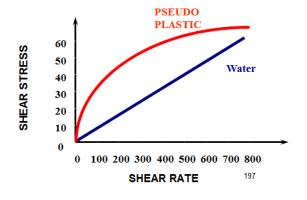
What is the exact reason why such a change of fluid properties are desirable in Hydraulic Fracturing?
