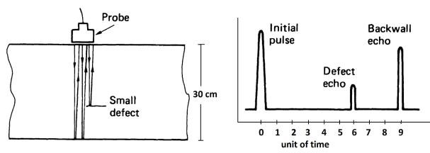
b) Using the same type of setup as shown in above image, ultrasonic inspection of a casting was carried out. Below figure shows the output screen display obtained. What kind of defects/flaws present in the casting could be responsible for it? (5)
