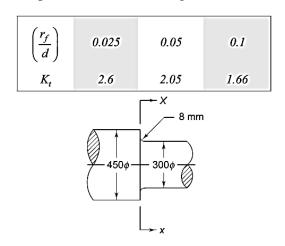
where  $r_f$  is the fillet radius and d is the shaft diameter. The reliability is 90% ( $K_c$ =.897).Determine the life of the shaft.
