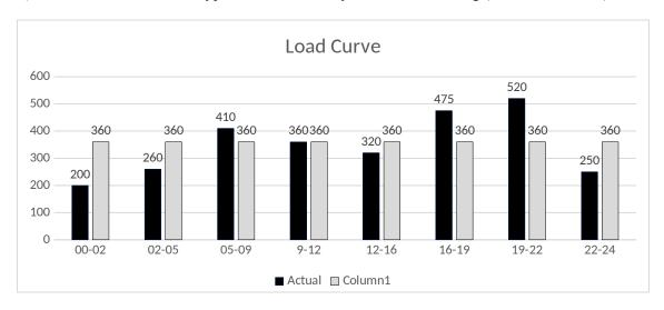
The DISCOM has to meet the peak demand and hence the company has to install a 520 MW power plant. But installing a 520 MW will be requiring a very huge investment (Appro. 2000 crores). Instead DISCOM propose to set up Smart Grid and average out load to 360 MW (Light gray colored bars) and install a Generating station of 360 MW (appro. 1600 Crore).
