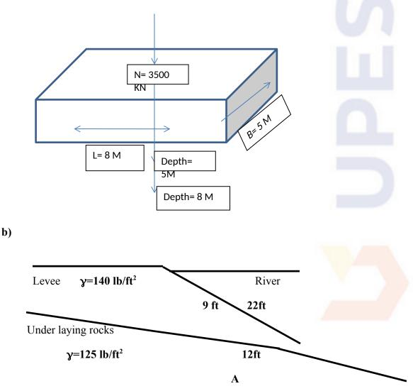
The above figure showing proposed levee is to be built along the side of a river to protect a nearby town from flooding. If the natural soils below the levee are clean sands with  $\phi = 34^{\circ}$  and the shear stress at point A is 555 lb/ft<sup>2</sup>. Determine the factor of safety against sliding at point A assume point A is nearly horizontal C<sup>-</sup>=0 5 M
