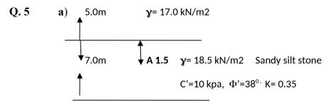
The series of shear strength test performed on above said lithology and calculated values are shown in the figure. Determine the shear strength on horizontal and vertical planes at point A for above given values. 6 M
