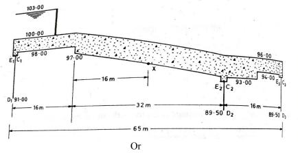
Design crest wall, cistern, impervious floor by Khosla's Theory for unflumed glacis non meter Fall for the following Data
