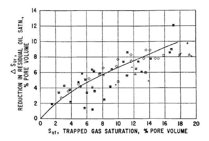
Figure-2: *Effect of*  $S_{gt}$  *on water flood recovery.*
