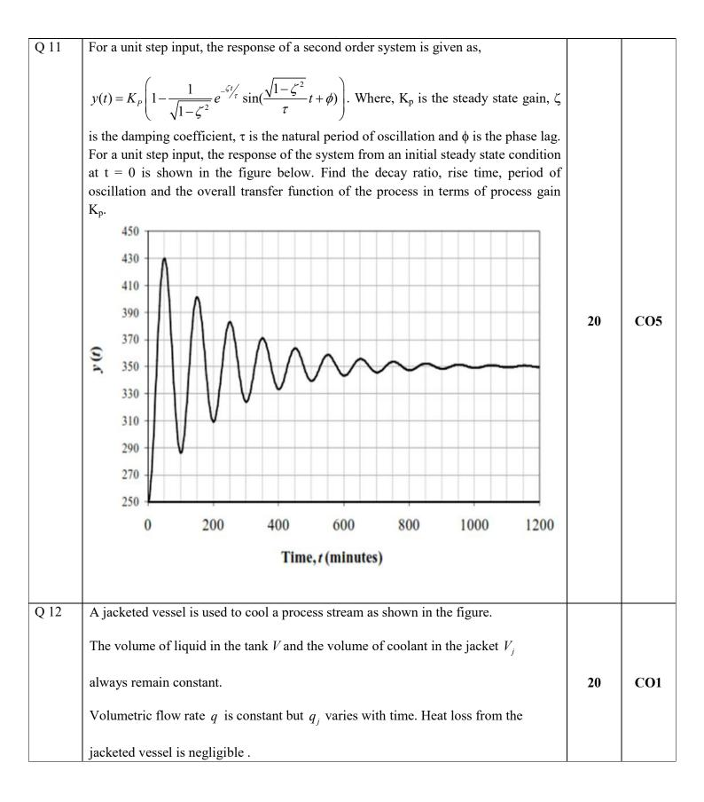
Both tank contents and jacket contents are well mixed and have significant thermal capacities. Thermal capacities of tank wall and jacket wall are negligible. The overall heat transfer coefficient for transfer between tank liquid and coolant varies with coolant flow rate,  $U = K q_j^{0.8}$ , Where K is constant. Derive a transfer function model for this system. (State any additional assumptions that you make.)
