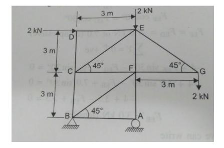
8. Find the method of joints of the forces in the members of the truss shown in figure:
