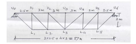
b) Two wheel loads 50 kN and 20 kN spaced 2m apart with load 20kN in the lead rolls on the girder shown in the figure. Use influence lines to determine the maximum (+ve & -ve) shearing force and bending moment at the section C. The load system can move in either direction. [CO3]
