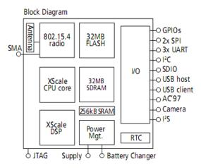
Figure 1: IMote2 Sensor Node Hardware
