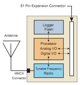
Figure 1: MICA2 Sensor Node Hardware
