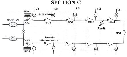
The figure represents a typical 11 kV distribution network section. IED1 & IED2 consists an over current protection element. The fault occurred in between SD3 and SD4. Restore the supply in less span time is the main objective. Considering the data given,
