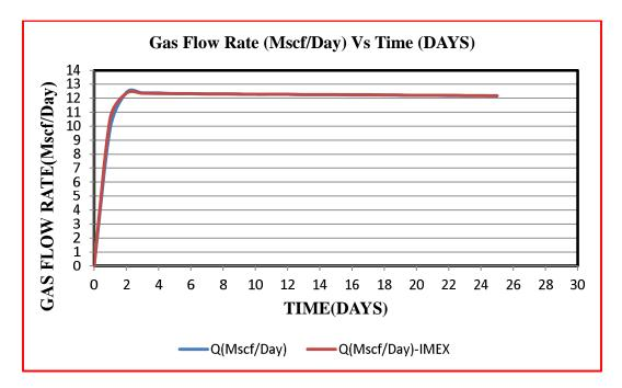
Figure 8.2: Variation of Gas Flow Rate (Mscf/Day) Vs Time (DAYS).
