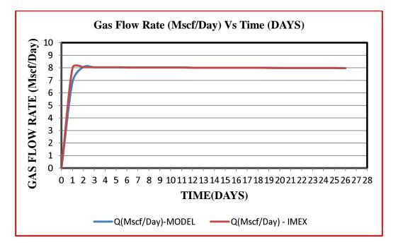
Figure 8.1: Variation of Gas Flow Rate (Mscf/Day) Vs Time (DAYS).
