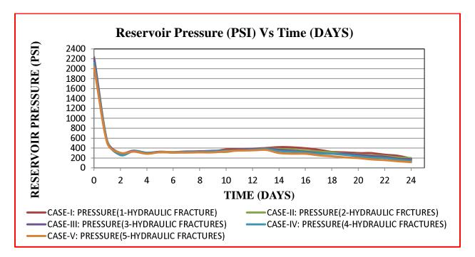
Figure 8.8: The pressure variations in reservoir versus time at different fracture stages.
