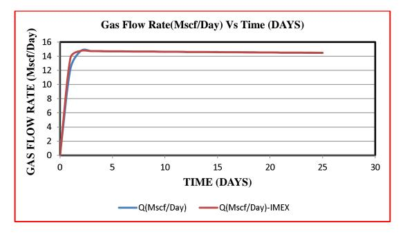
Figure 8.3: Variation of Gas Flow Rate (Mscf/Day) Vs Time (DAYS).
