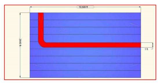
Figure 5.1: Shale reservoir with horizontal wellbore and no hydraulic fractures.
