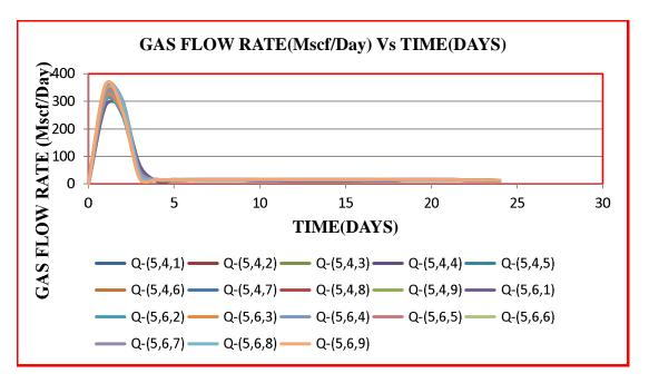
Figure 5.3, represents the rate of flow of gas from the matrix block in the horizontal wellbore.
