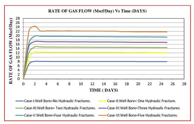
Figure 5.7: Gas flow rate variation with time at different Hydraulic Fracture Stages.
