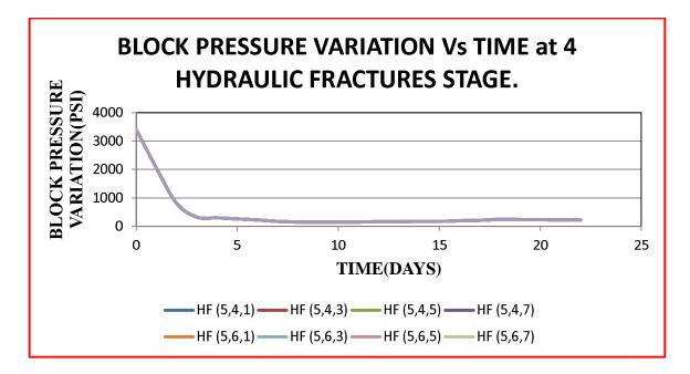
Figure 5.5: Pressure variation at different block of hydraulic fractured zone with respect to time.
