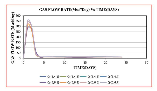
Figure 5.6: Gas flow rate variation with respect to time in different fractured blocks.
