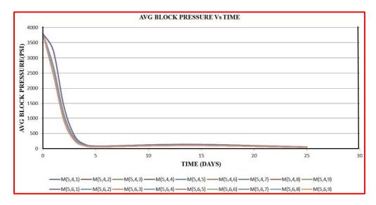
Figure 5.2: Individual matrix block pressure variation with time.
