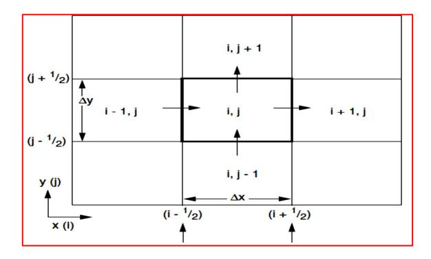
*Figure 4.2: Discretization and notation indication for a 2D pressure equation for Matrix.* By applying finite difference method to equation 7, we get
