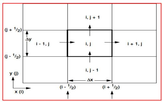
*Figure 4.3: Discretization and notation indication for a 2D pressure equation for Hydraulic Fracture.*
