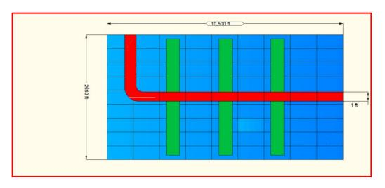
*Figure 4.3(c): Schematic Representation of a Three Hydraulically Fractured Reservoir.*
