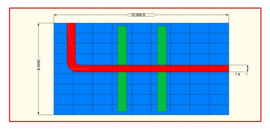
Figure 4.4(b): Schematic representation of a Two Hydraulically Fractured Reservoir.
