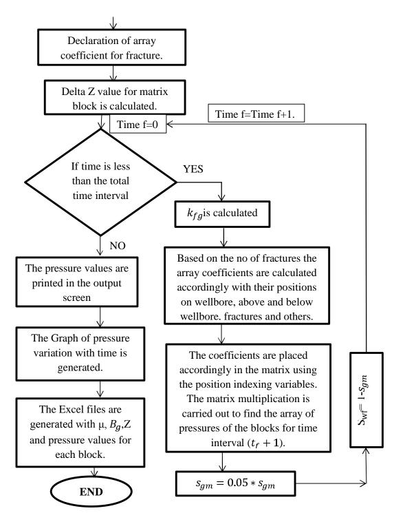
*Figure 4.5: Algorithm representing the procedure for solving the gas flow in the hydraulic fractures.*
