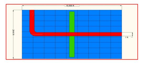
*Figure 4.4(a): Schematic representation of a Single Hydraulically Fractured Reservoir.*
