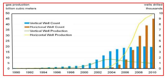
Figure 1.4: Increase in production and well count in the Barnett shale from 1990 to 2010 (Newell, 2010).
