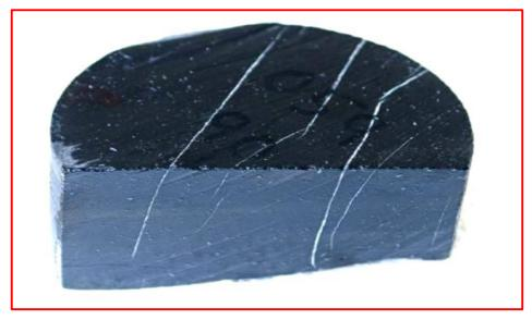
Figure 1.6: Core Sample from Barnett Shale (Bowker, 2013).
