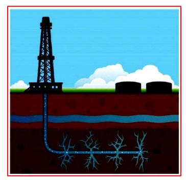
Figure 1.7: Horizontal drilling and multi-stage hydraulic fracturing (Web Page)
