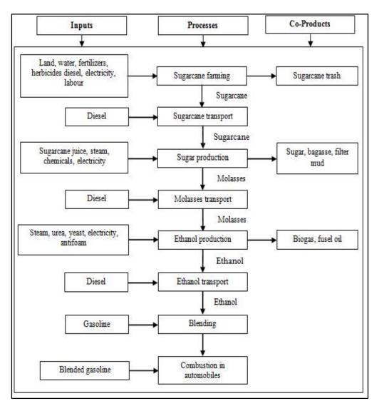
Figure 4.3 System boundaries for the 1G fuel ethanol production in India
