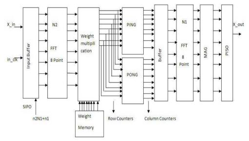
Fig.3.10. Internal Block diagram of the 64-point FFT module
