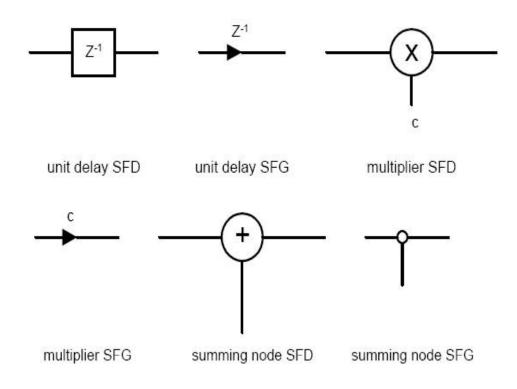
Fig.3.1. Symbols used in Digital filter structures.
