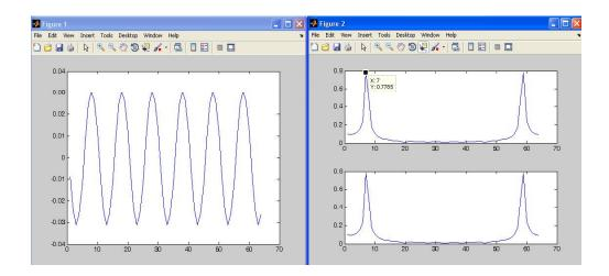
Fig.3.11. FFT 64 with two 8 point FFTs MATLAB results
