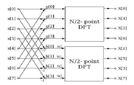
Fig.3.2. First stage of 8-point Decimation in Frequency FFT algorithm
