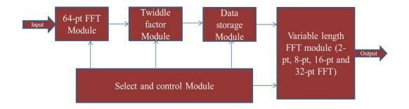
Fig.3.8.Block diagram of the overall design of the Variable length FFT processor
