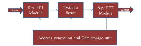
Fig.3.9. Pipeline structure of 64-point FFT Processor
