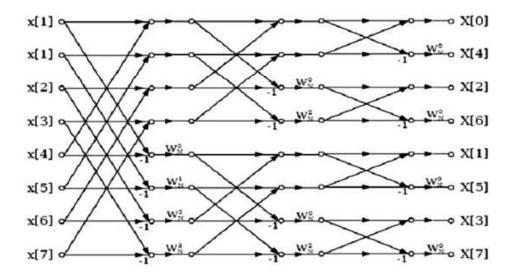
Fig.3.4 Structure of 8-point Decimation in Frequency FFT algorithm
