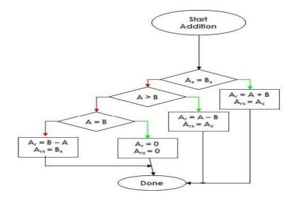
Fig 3.5.Flowchart of Addition and Subtraction with Signed-Magnitude Data
