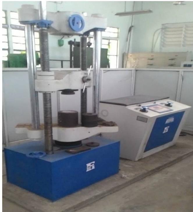
**Figure 3.6: Universal testing machine**
