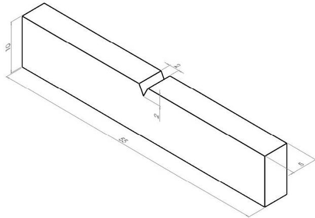
**Figure 3.8: Standard specimen for Impact test**
