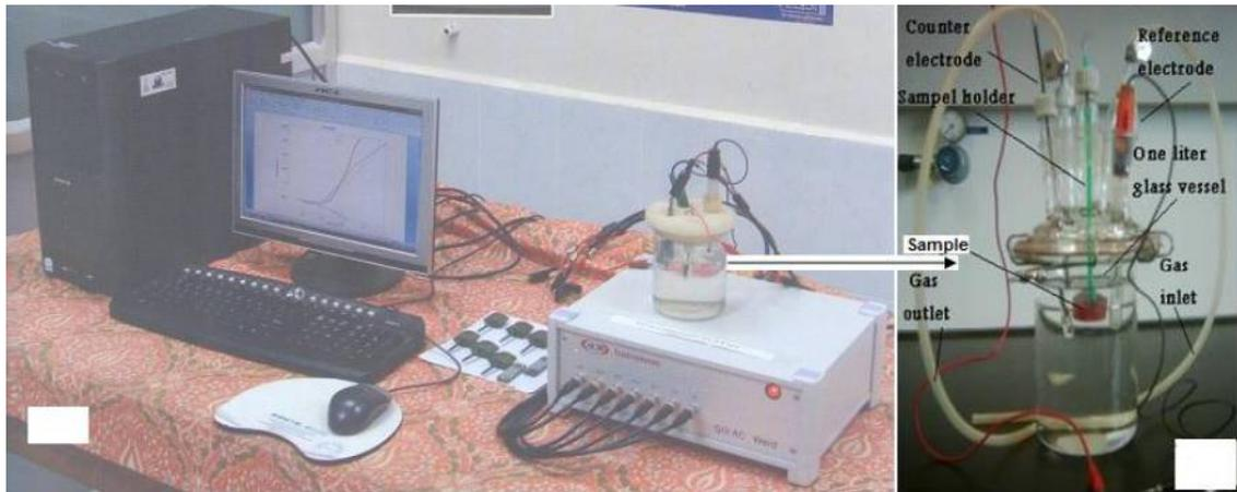
**Figure 3.5: Corrosion testing setup**
