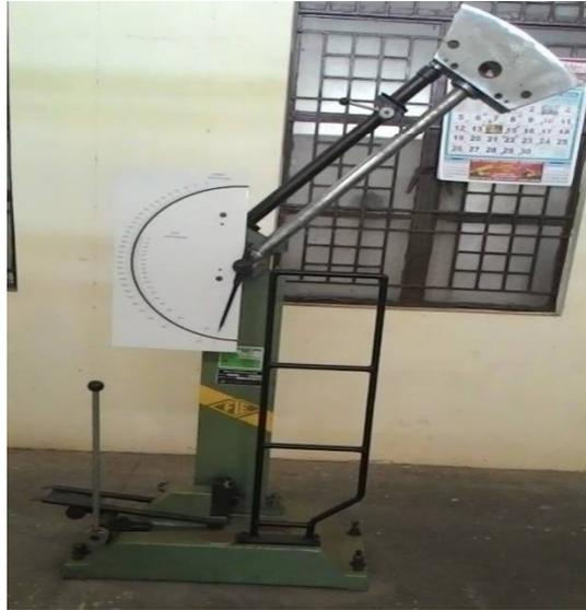
**Figure 3.7: Impact testing machine**
