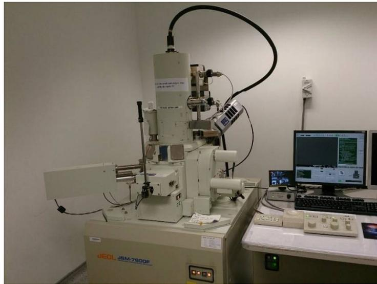
**Figure 3.3: SEM-EDS equipment**
