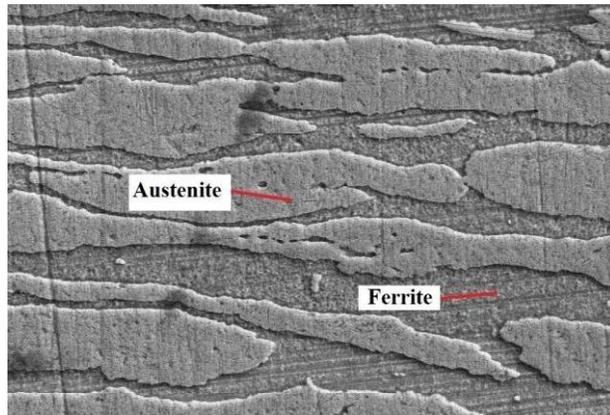
**Figure 3.1: Typical base material microstructure**
