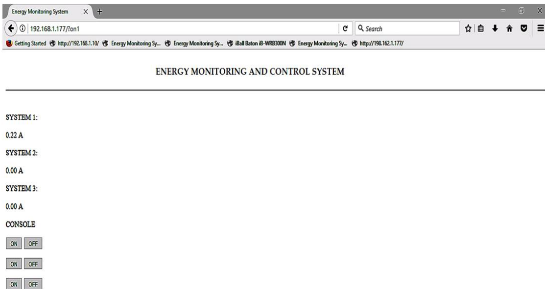
Fig.5.13. Snapshot of remote wireless monitoring and control of smart power system through HTML webpage
