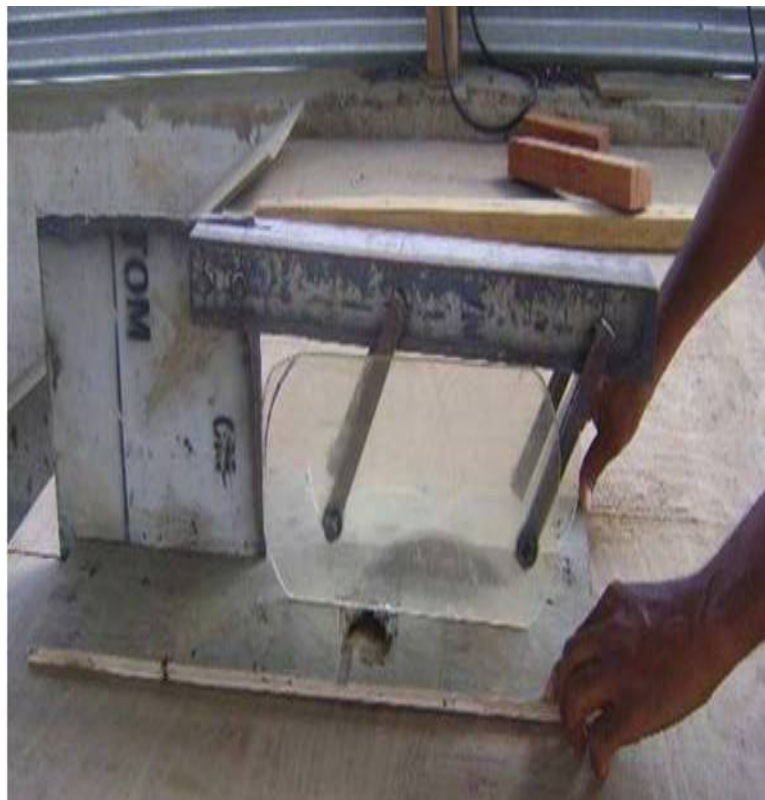
Type V: Circular saw guard with flap type acrylic material
