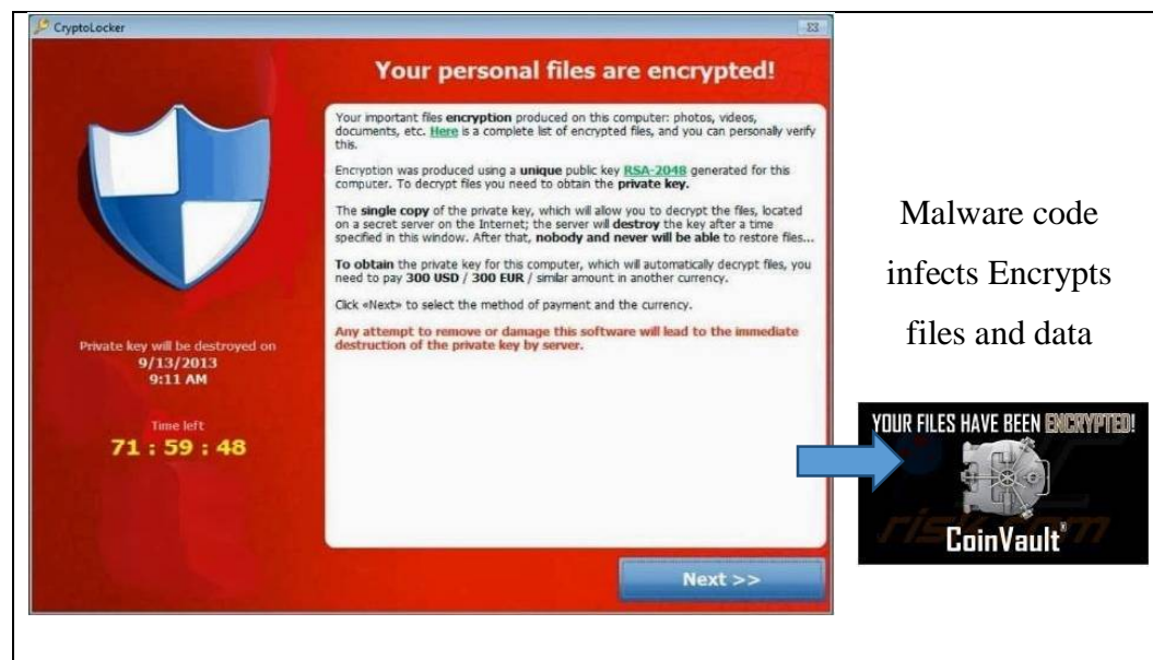
Figure 1.15: Crypto Ransomware Data Encryption
