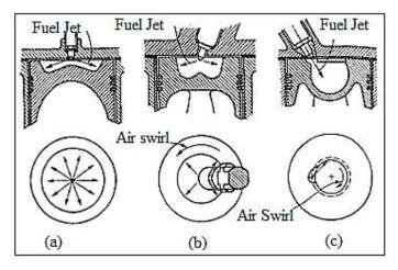
Figure 1.3 Common types of Combustion Chambers of Direct Injection Systems (a) quiescent chamber with multi-hole injector for large size engines (b) bowl- in –piston chamber with swirl and multi hole nozzle for medium to small size engines(c) bowl- in –piston chamber with swirl and single hole nozzle for medium to small size engines [3]
