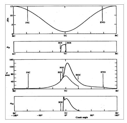
Figure 1.2 Sequence of compression, combustion and expansion processes of a naturally aspirated compression ignition engine [3]
