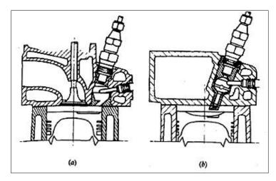
Figure 1.4 Common types of Combustion Chambers in IDI engines (a) Swirl pre-chamber (b) Turbulent pre-chamber [3]
