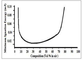
Figure 1.8 Minimum Ignition energy of H<sub>2</sub>-Air mixture
