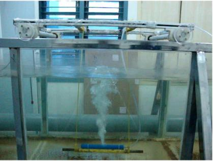
Fig 5.14: Plume behaviour atDepth: 1mFlow Rate: 0.0112m³/s
