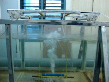
Fig 5.13: Plume behaviour atDepth: 1mFlow Rate: 0.00758m³/s
