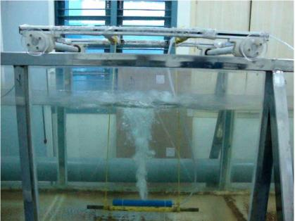
Fig 5.12: Plume behaviour atDepth: 1mFlow Rate:  $0.00505m^3/s$
