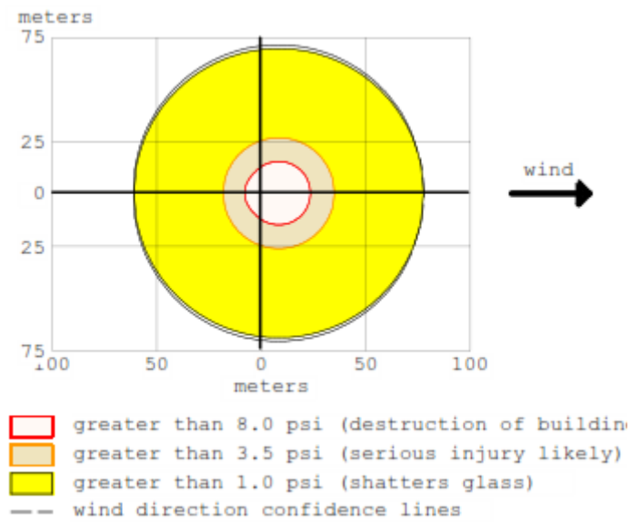
Figure 4.18 Pressure danger zones
