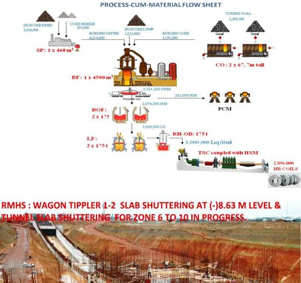
Figure - 1.1: Typical Process-cum-flow sheet of a Steel Plant
