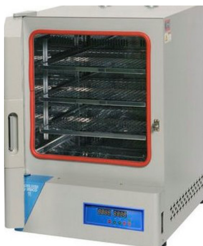
Figure 3.7: Furnace, which is used for catalysts drying
