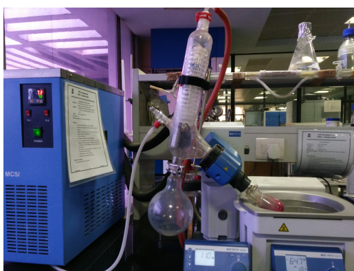
Figure 3.5: Removal of solvent from the catalyst using Rotavapor
