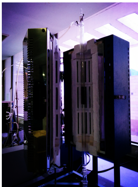
Figure 3.8: Catalysts inside tubular reactor in calciner
