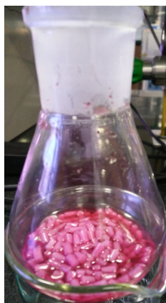
Figure 3.4: Impregnated CP Catalyst supported on \text{SiO}_2 (standing at room temperature for 140 mins)
