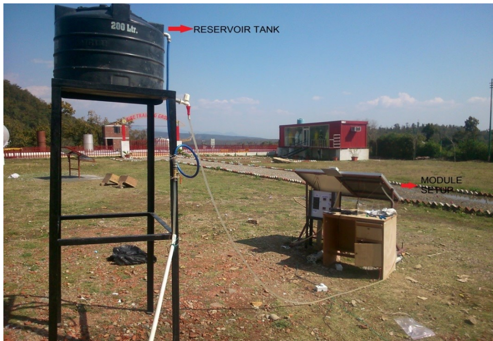
Fig 3.9: Prototype reference and modified PV panels installed at experiment site
