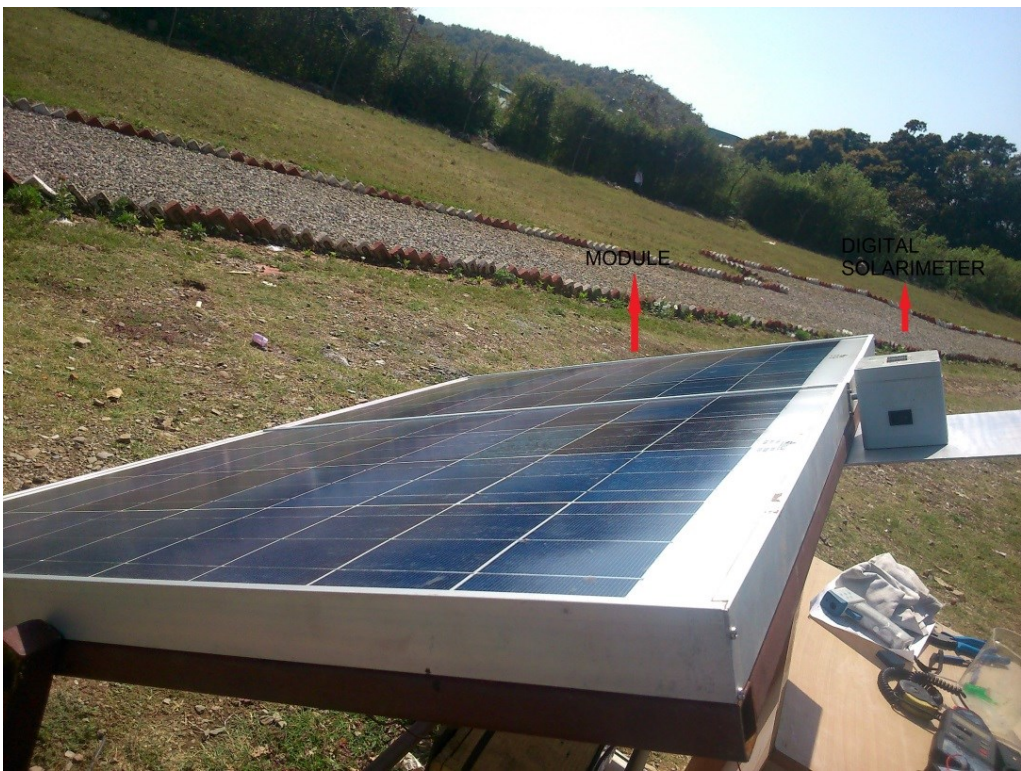
Fig 3.5: Measurement of solar radiation on tilted surface
