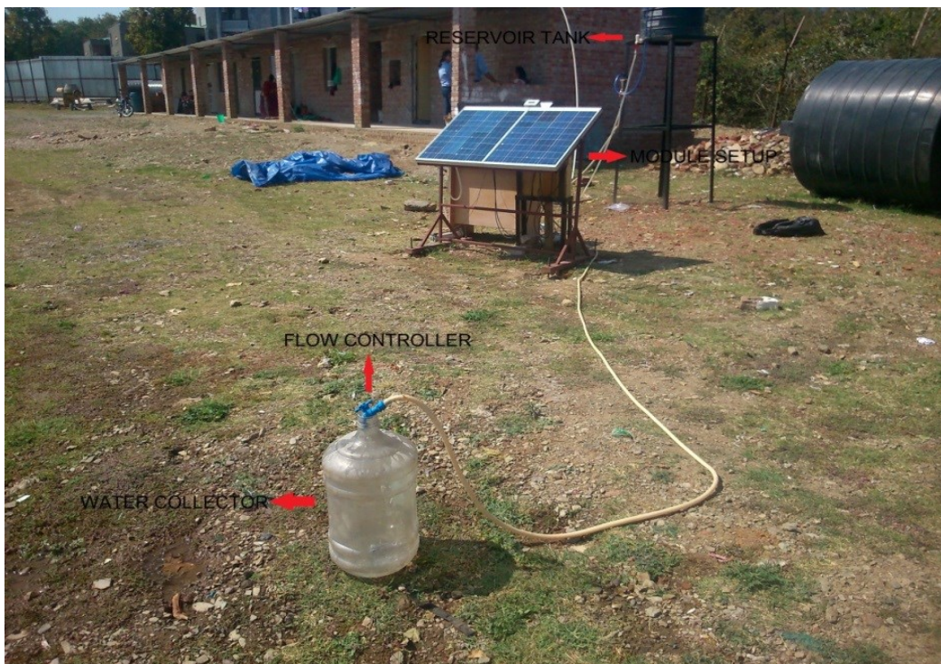
Fig 3.7: Mechanism to set water flow rate
