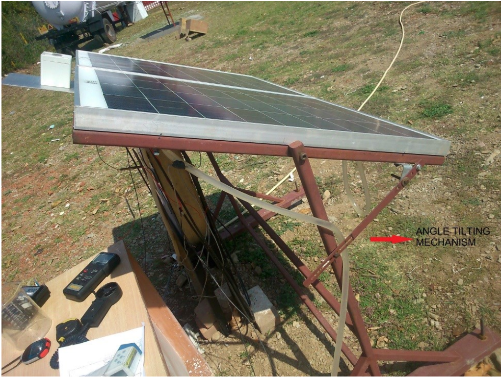
Fig 3.4: Angle tilting mechanism
