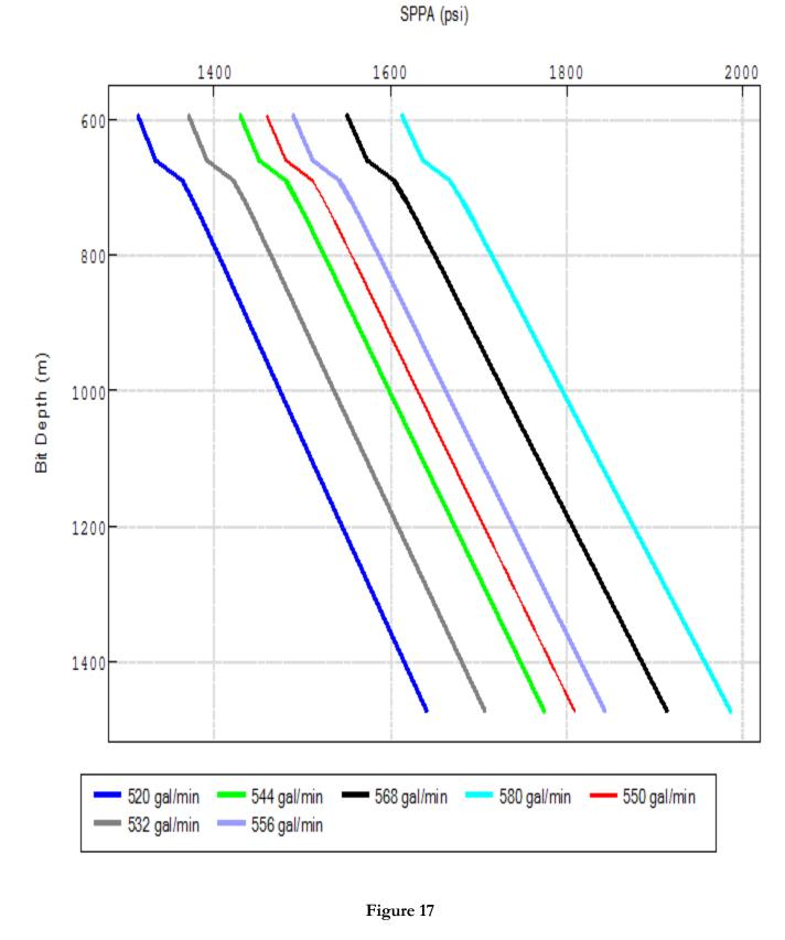
The plot of standpipe pressure and it's variation with depth at different flow rates is plotted.
