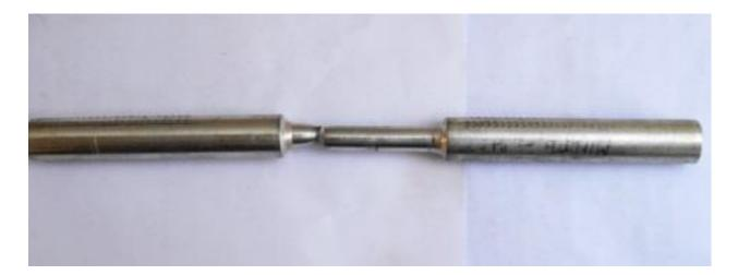
Fig 16: Zinc Coated UTM Test Specimen
