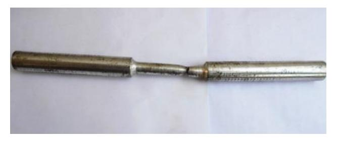
Fig 17: Zinc Coated Corroded UTM Test Specimen
