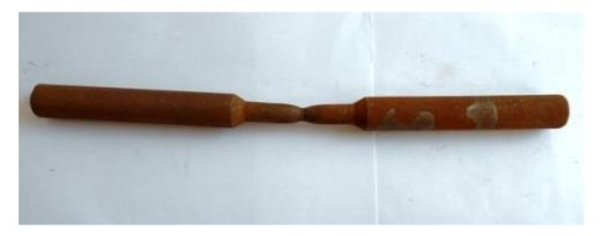
Fig 15: Bare Corroded UTM Test Specimen
