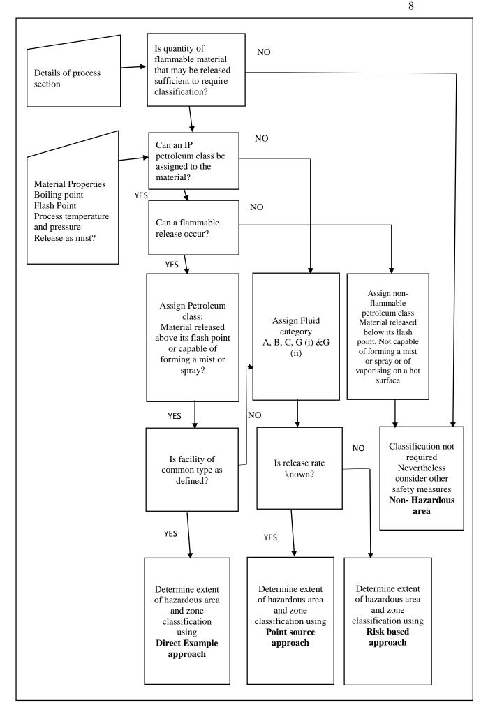
Figure 3.1: Hazardous Area Classification Methodology (IP-15)
