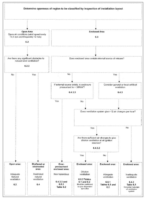
Figure 3.2: Procedure for assessing type and degree of ventilation (IP-15)
