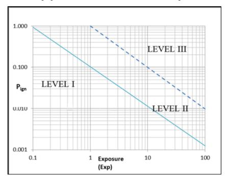
FIGURE 3.4: Release frequency Level Graph (IP-15)
