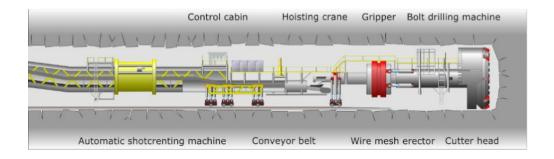
Figure 1.3: Tunnel Boring Machine
