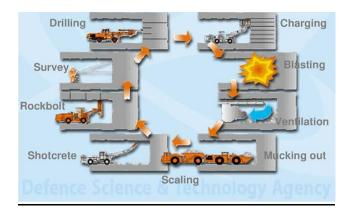
Figure 1.4: Tunneling life cycle
