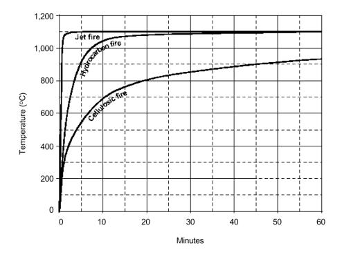
**Figure 4.2 - Time–Temperature Curve for Fire Tests**
