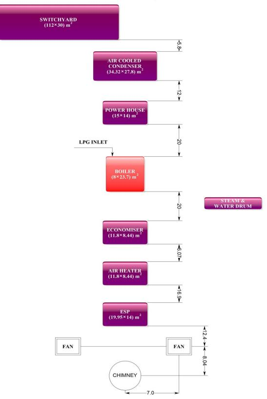
**Figure 3.3 – Co-Generation Equipment Layout**
