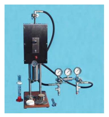
**Figure 22 - HTHP filtration test**
