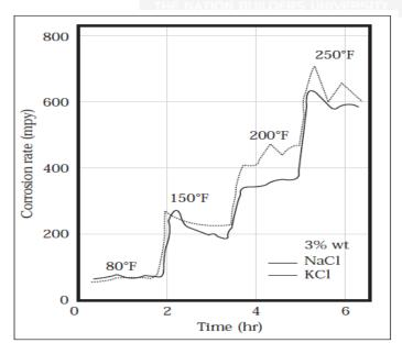
Figure 11 - The rate of corrosion changes temperature & pressure
