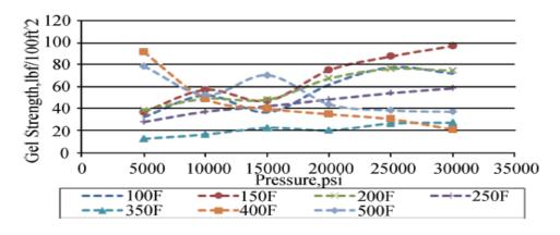
Figure 6 - Gel strngth changes with temperature & pressure
