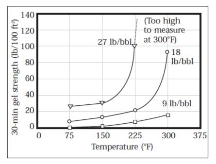
Figure 7 - 30 min gel strength changes with temperature
