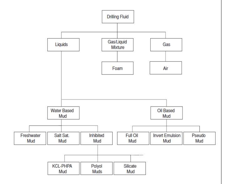
Figure 1 - Types of drilling fluid
