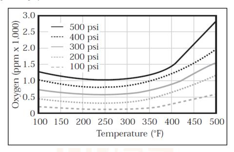
Figure 10 - solubility of oxygen changes temperature & pressure
