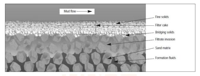
Figure 8 - A Thin, lower permeability mud filter cake
