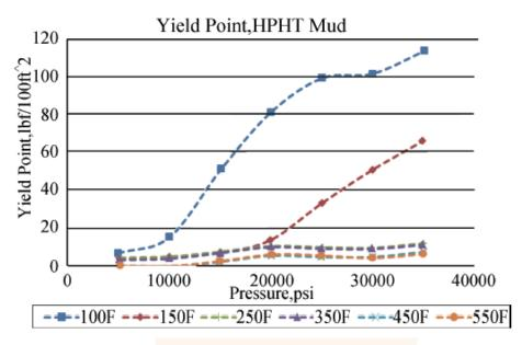
Figure 4 - yield point changes with temperature & pressure
