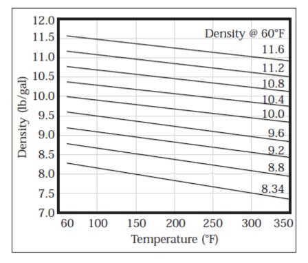
Figure 3 - Density changes with temperature
