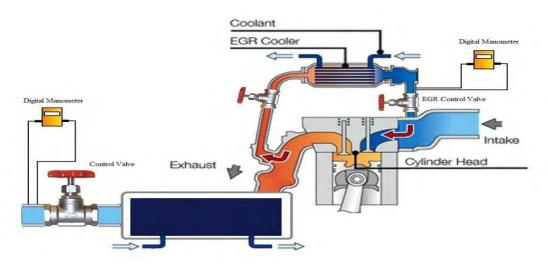
Figure 1. A schematic diagram of EGR system
