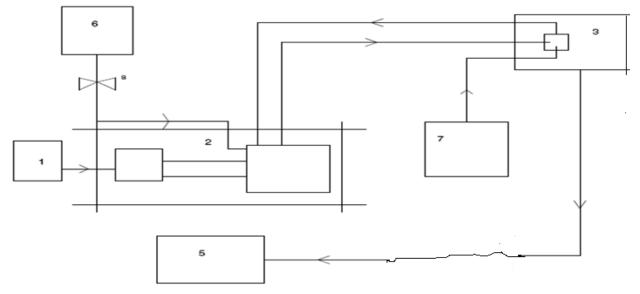
1. Electrical loading 2. Single cylinder 4-stroke diesel engine & Alternator 3. Exhaust gas recirculation system 5. Gas Analyzer Smoke meter 6. Fuel Tank 7. Air drum 8. Control valve
