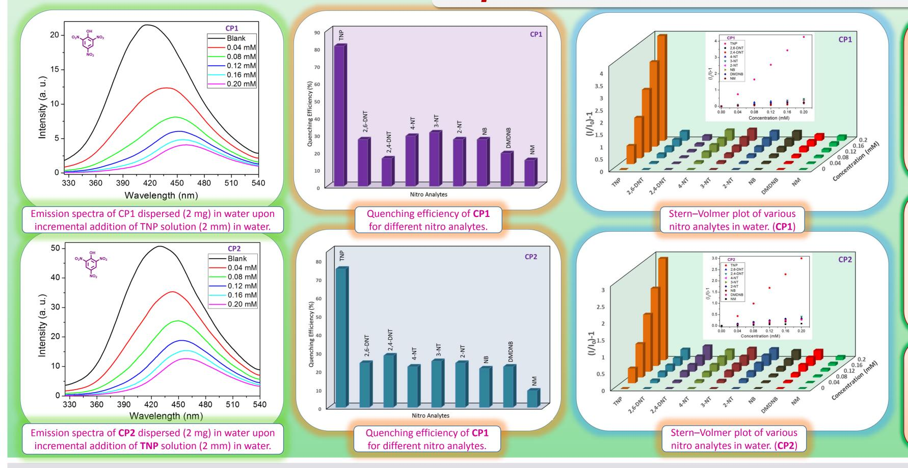
**Experiment:** As synthesized CPs were added to a fluorescence cuvette containing 2 mL water. Emission ( $\lambda_{ex} = 295$  nm) was measured in 325-540 nm range *in-situ* after incremental addition of freshly prepared aqueous nitroanalyte solutions (2 mM). The solution was continuously stirred throughout the experiment. Triplicate experiments yield consistent results.
