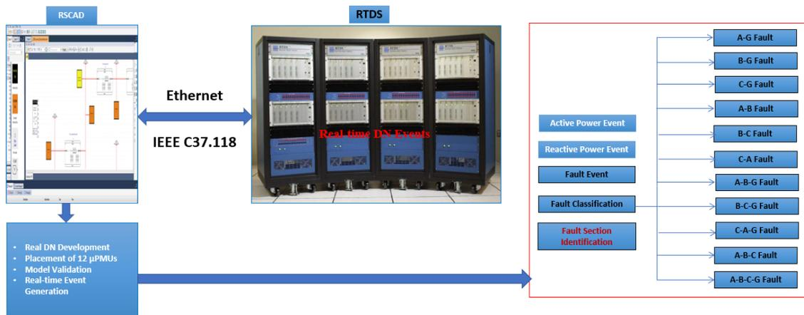
FIGURE 6.57: RTDS testbed for generated data validation
