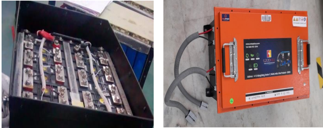
Fig. 4.15 LFP battery pack actual view (a) battery pack with top cover opened, (b) battery pack ready for assembly with e-mobility.
