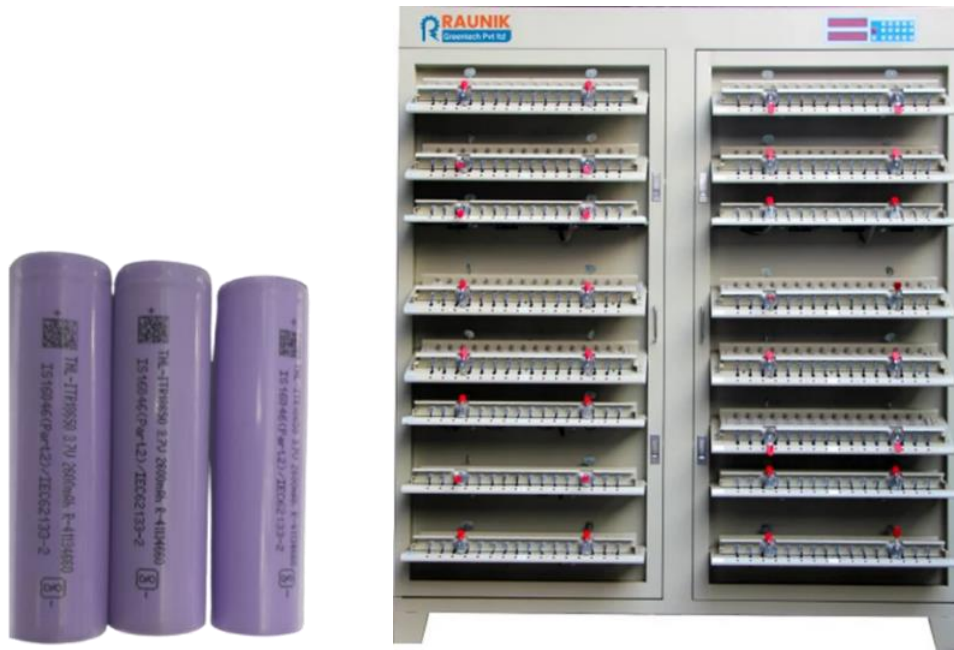
Fig. 4.4 (a) Experimental cells (b) 512 cell grading machine for cell preconditioning test.
