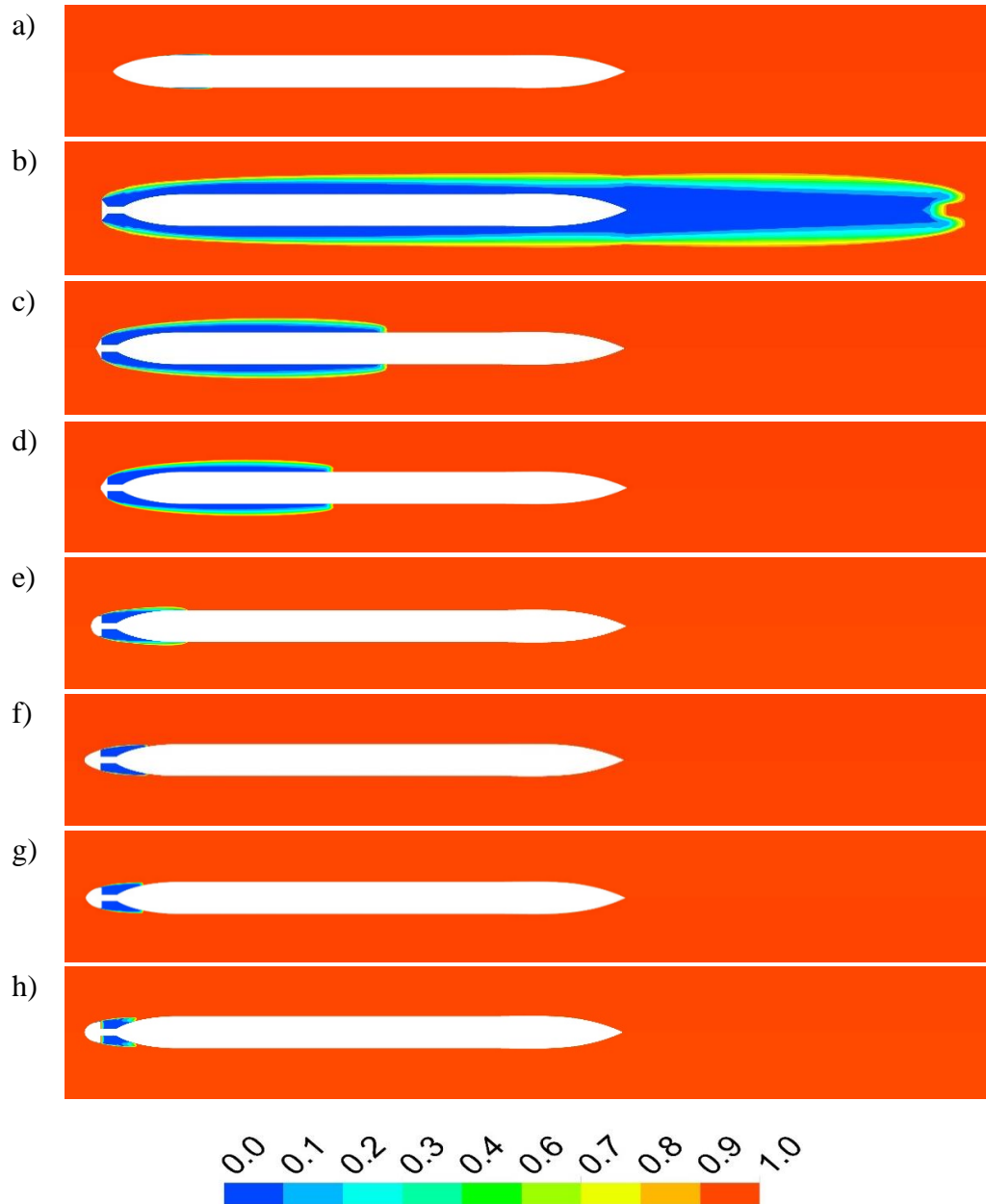
Fig. 3.9: Contour of volume fraction of seawater at \sigma_c of 0.09 for various cavitators: a) Without cavitator, b) DC, c) CC-120, d)TC-16, e) SC, f) PC g) MC-1.5, and h) EC
