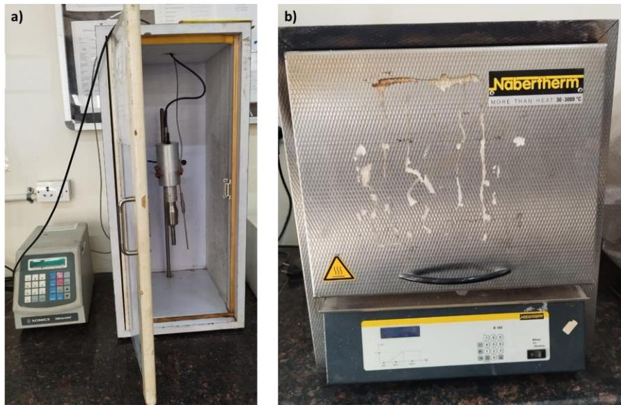
Figure 3-2: Images of Instruments used in setup a) Ultrasonicator (Sonics & Materials Inc., vibracell VCX -750) b) Programmable muffle furnace Nobertherm, 30-3000 °C
