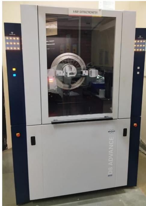
Figure 3-10: XRD setup, Bruker D8 ADVANCE ECO
