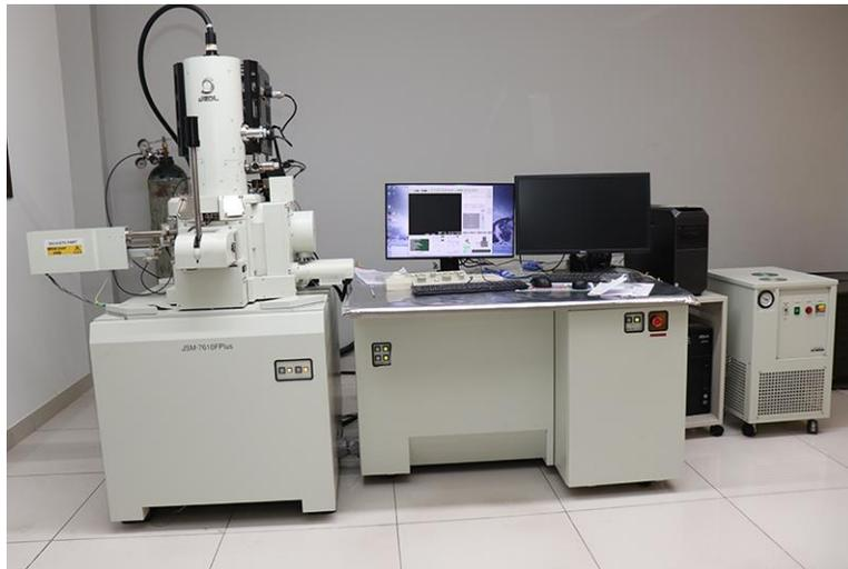
Figure 3-11: FESEM setup, JEOL make JSM-7610 FPlus, 1 kV 1.0 nm, 15 kV 0.8 nm
