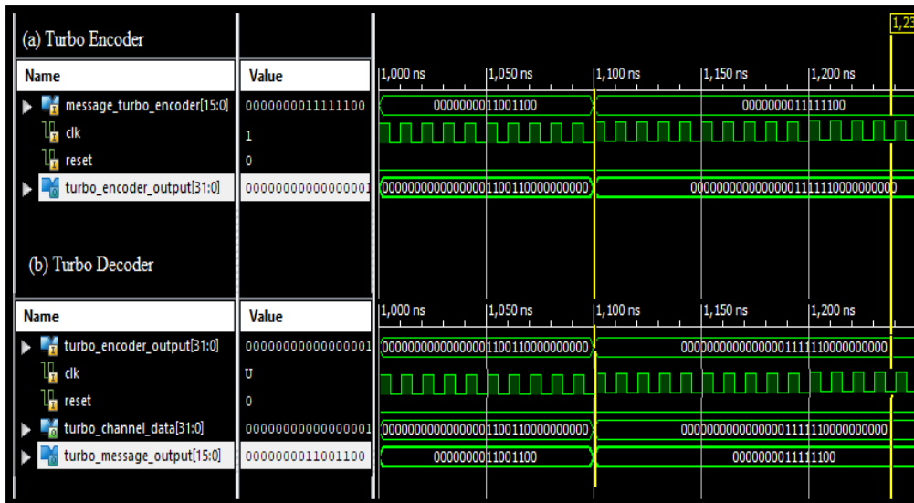
Fig.6.20 Xilinx ISIM simulation for Turbo encoder and decoder
