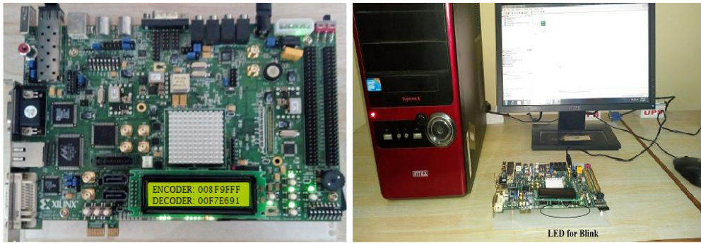
Fig. 6.41 FPGA logic verification
