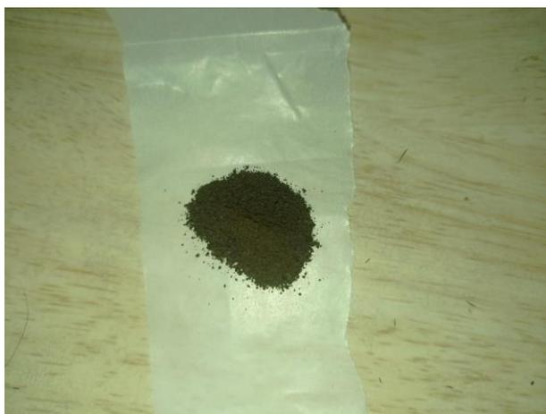
*Fig.13 :  $\text{NiFe}_2\text{O}_4$  powder*
