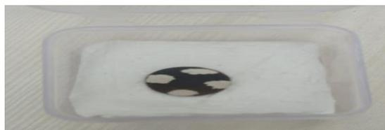
*Fig12: r-Go doped Fe<sub>3</sub>O<sub>4</sub> Pellet*
