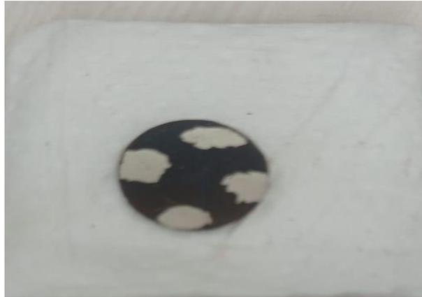
*Fig15: Palletisation r-GO dopped Fe<sub>3</sub>O<sub>4</sub> nano particles*
