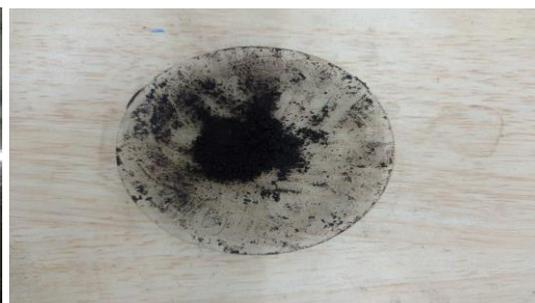
*Fig 11: r-GO doped Fe<sub>3</sub>O<sub>4</sub>*
