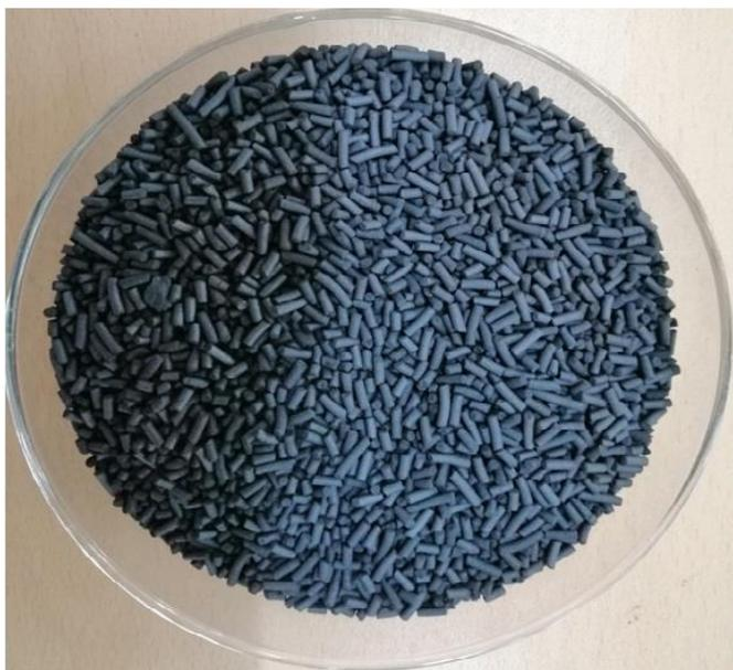
**Fig. 4.1** Commercial activated carbon Norit RB-2
