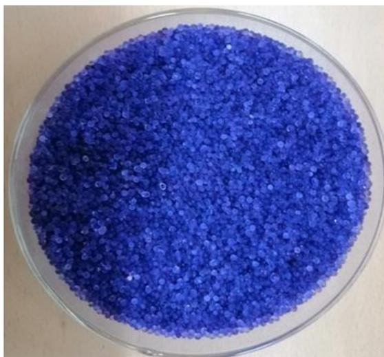
**Fig. 4.16** Silica gel type-III used for adsorption investigation
