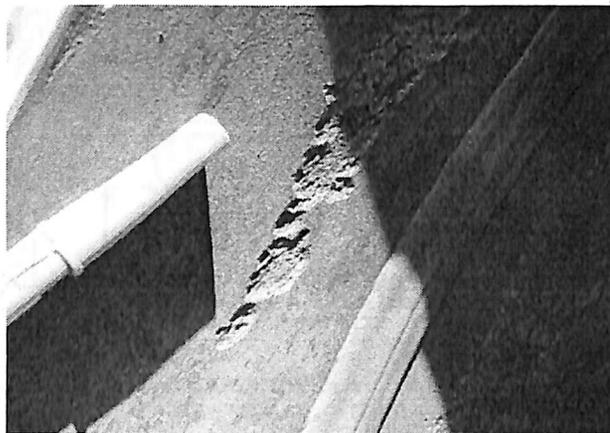
Figure 4: Chevron Refinery CDU. Severe Corrosion of Exchanger Channel (5 Cr- ½ Mo) Side Cut @ 650°F (343°C) [42]
