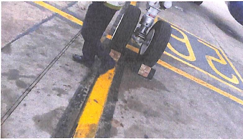
**Figure 1: placing the chocks.**
