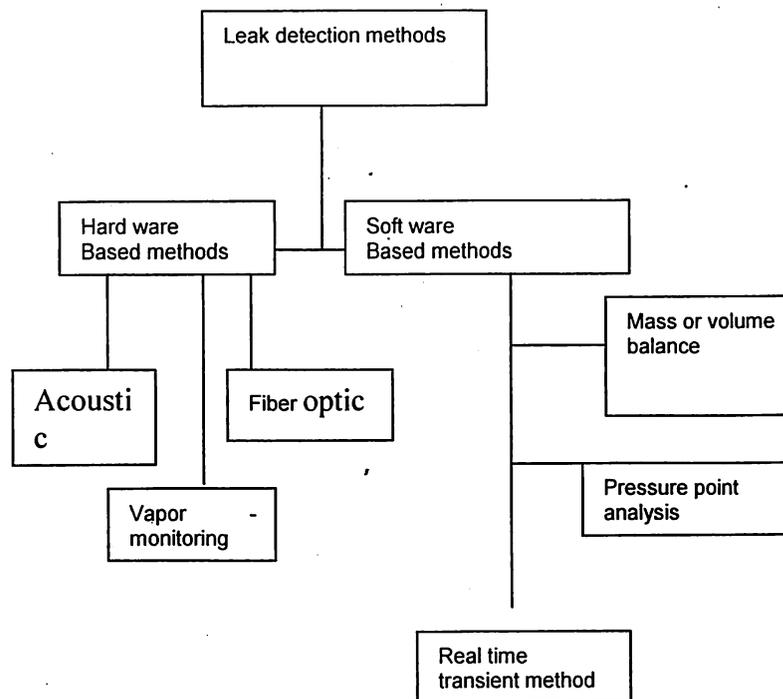
*Fig 3 CATEGORIZATION OF LEAK DETECTION TECHNOLOGY*
