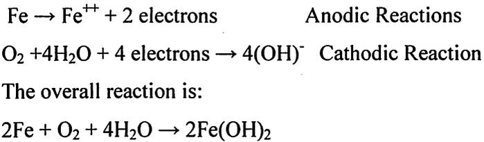
The higher the availability of the oxygen to the metal surface, the higher the potential rate of corrosion. Oxygen access to bare metal surface increases as the temperature of the water decreases or as the flow rate over the surface increases. Pipelines are, therefore, at high risk of corrosion in cold water moving at high velocity.
