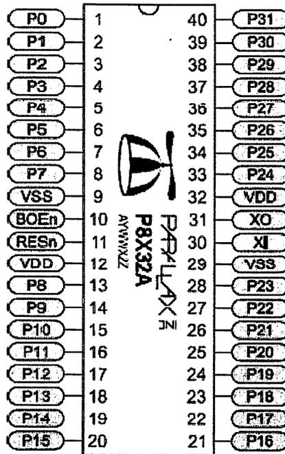
Figure 4.20: Parallax Microcontroller P8X32A-D40 40-pin DIP
