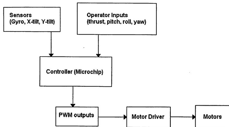
Figure 5.3: Control system schematic
