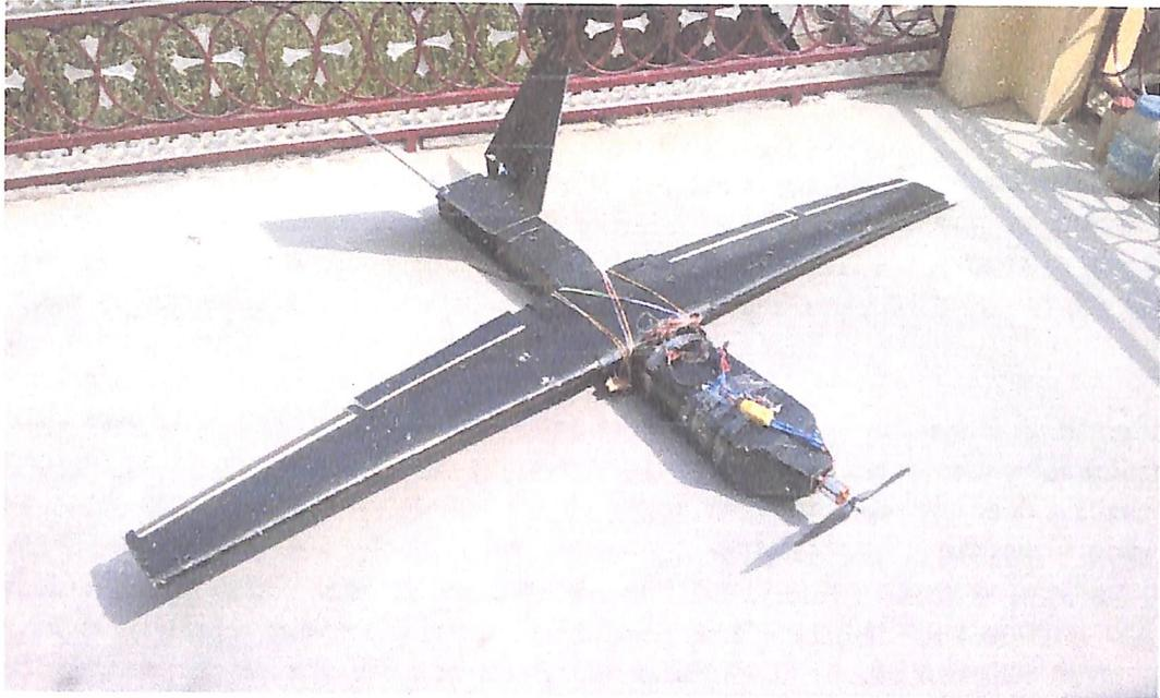
Figure 4.16: Complete prototype model of UAV
