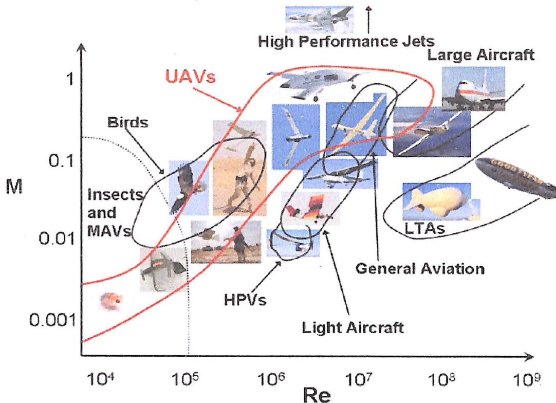
Figure 1.3: M versus Re for a wide range of airborne object
