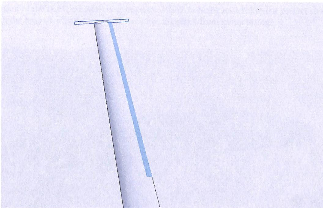
Figure 4.12: Extrude cut feature for attaching Ailerons
