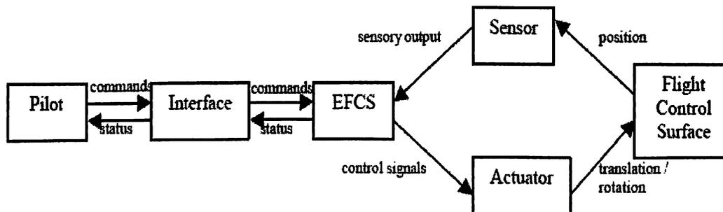
Figure 5.1: System top-level functions of the Flight Control System
