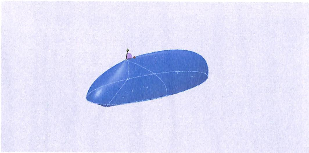
Figure 4.4: Extruded (with draft) Forward Cabin Structure
