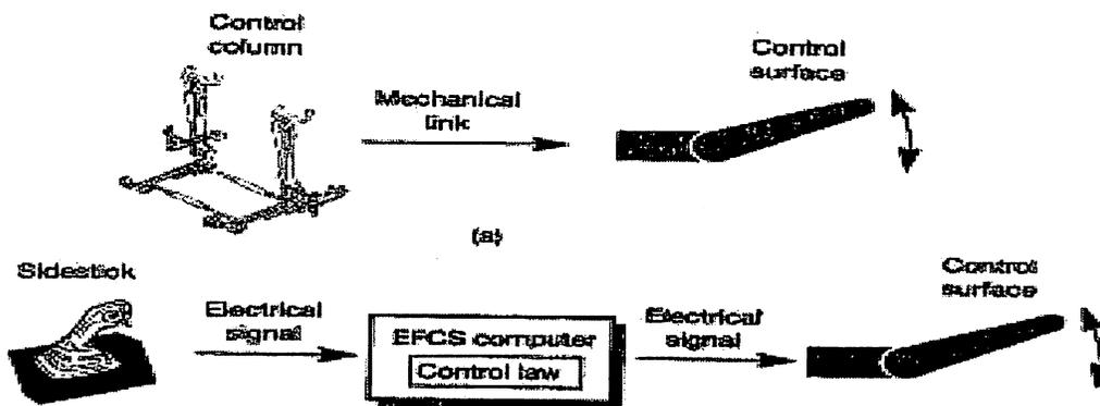
Figure5.2: Mechanical and Electrical control
