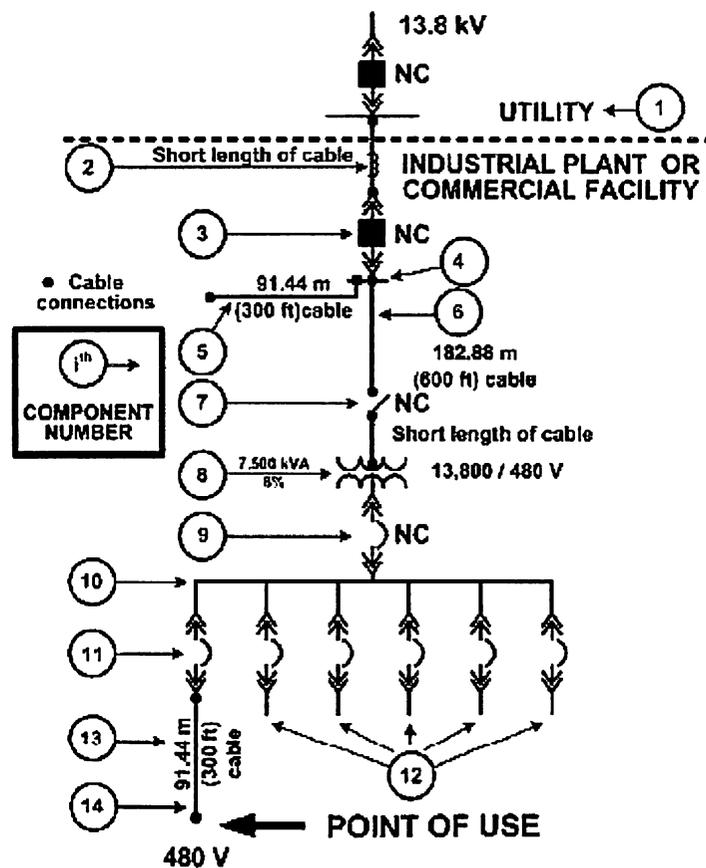
Figure-4.3- Simple radial system (Example-1)
