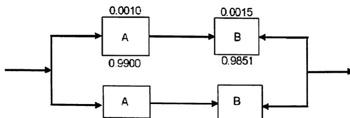
Figure-3.6.: RBD of a system with redundant components
