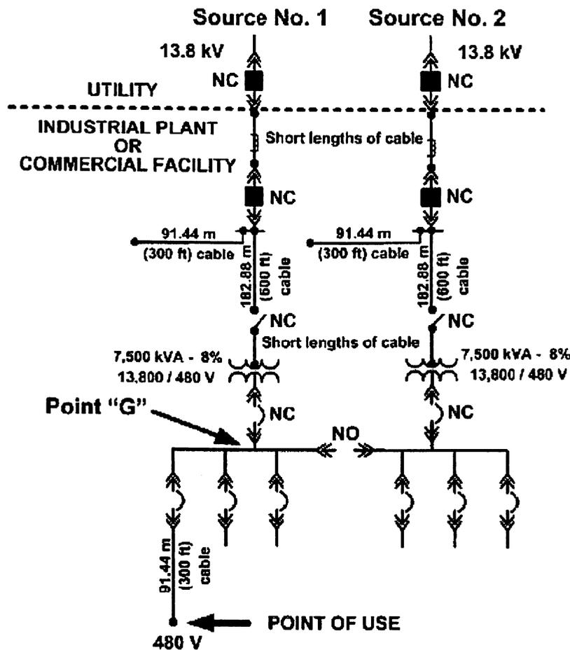
Figure-4.7 - Secondary-selective system (Example-5)
