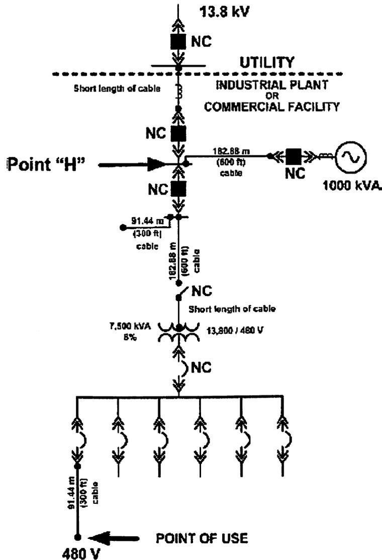
Figure 4.9 - Simple radial system with cogeneration (Example-7)
