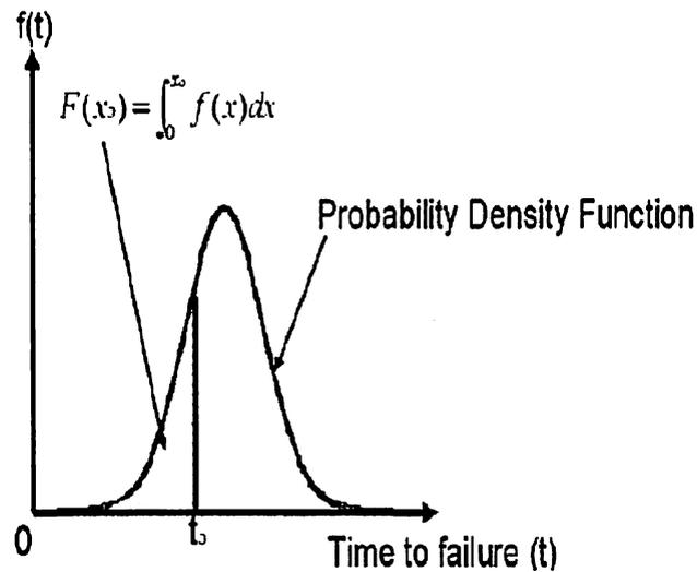
Figure-3.2: Probability of a failure represented by the area under the curve of the PDF
