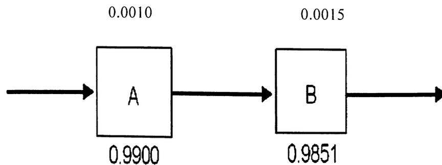
Figure 3.5: Example reliability block diagram
