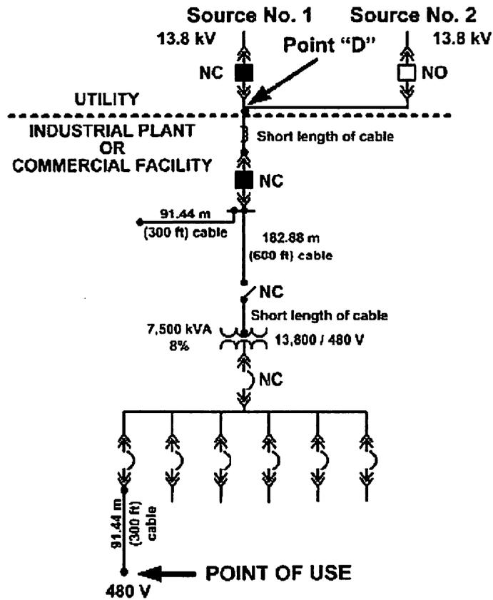
Figure-4.4- Primary-selective system to 13.8 kV utility supply (Example2)
