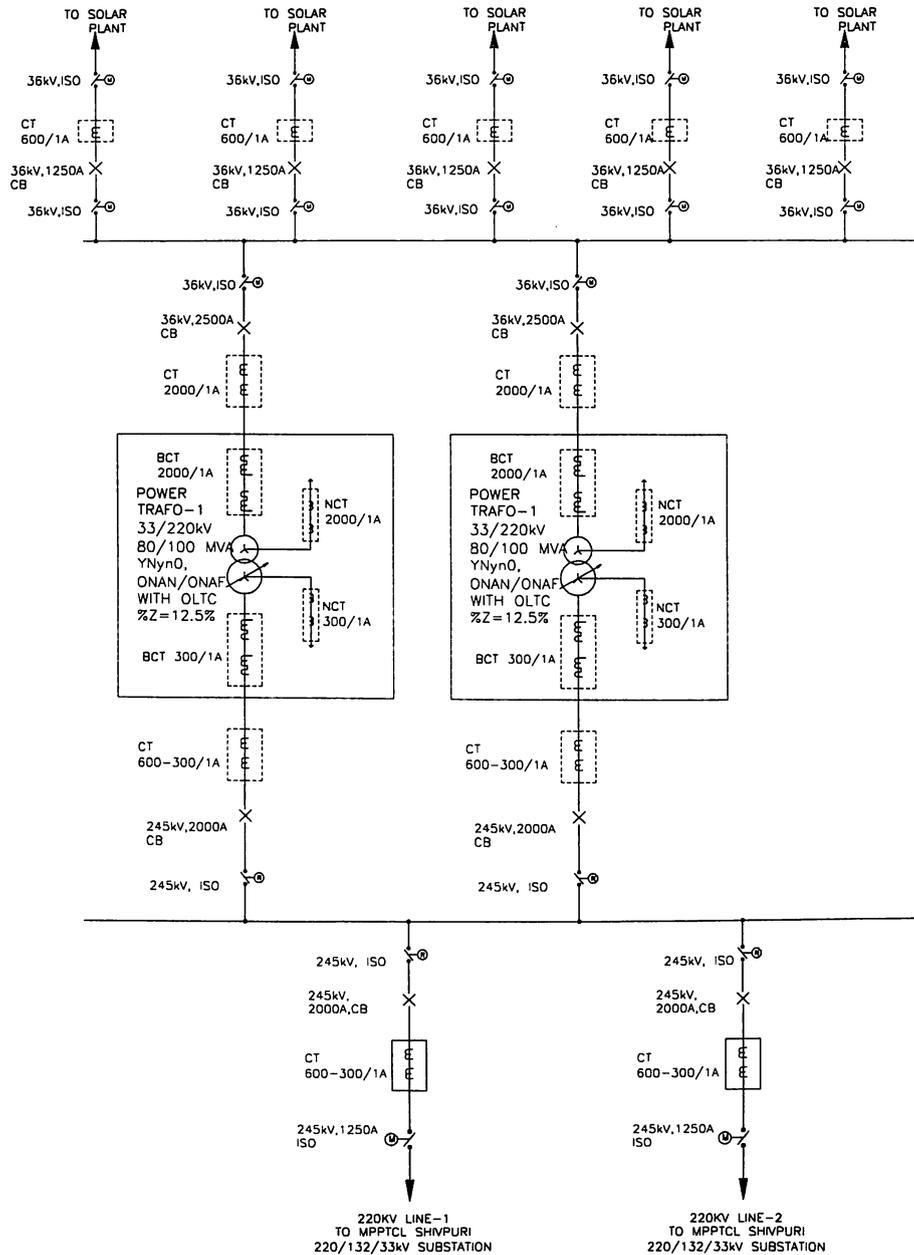
Fig-5.2: Single line diagram of 180MW substation proposal-2
