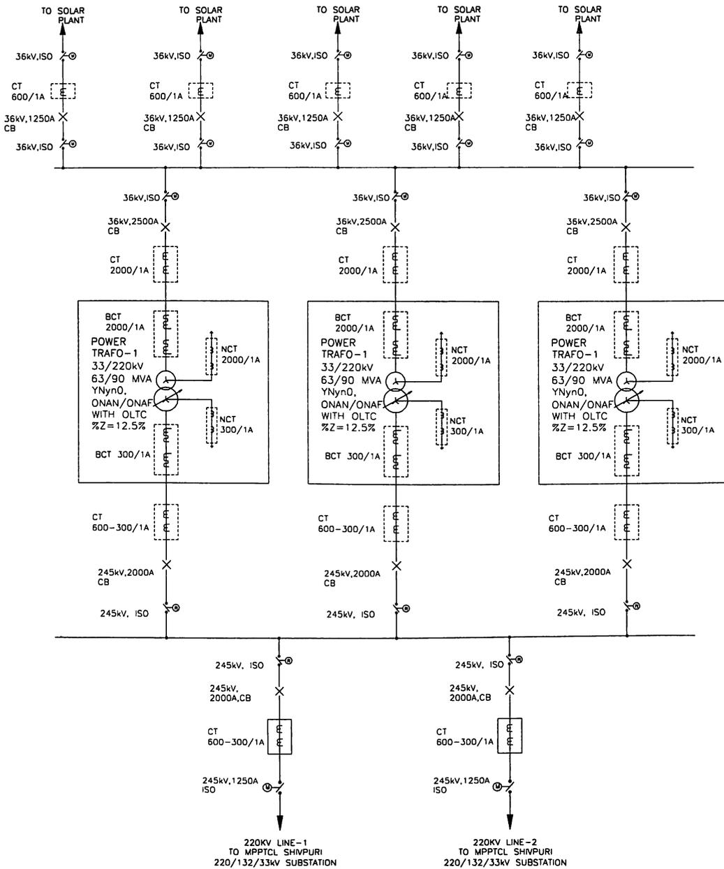
Fig-5.1: Single line diagram of 180MW substation proposal-1.
